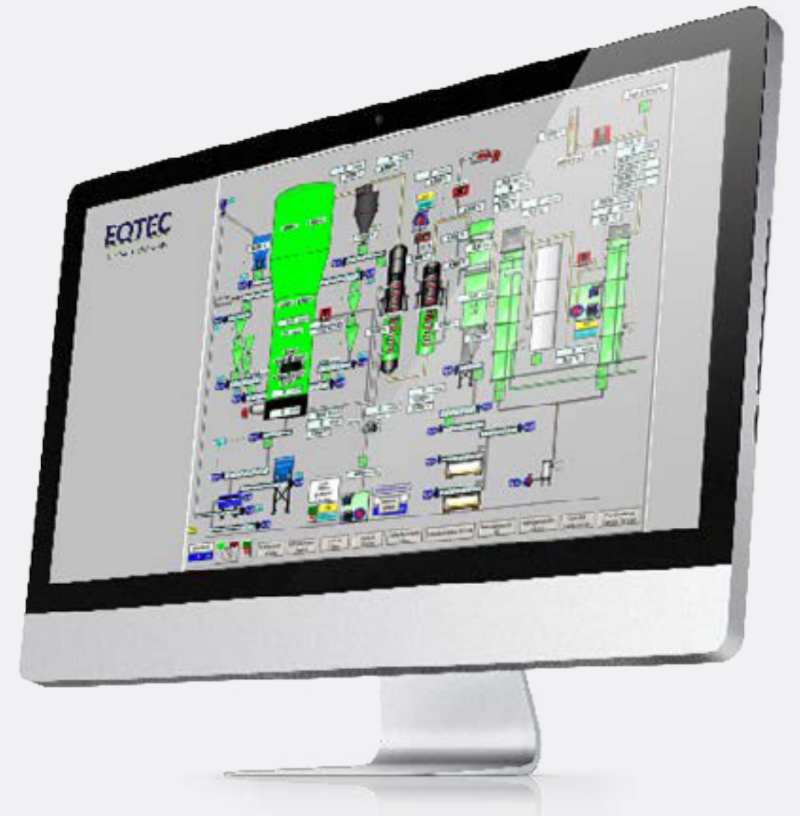
Images of the monitoring system a waste gasification plant industrial agriculture, with indication of the main operating variables.
